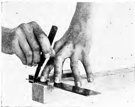
Fig. 65—Setting Try-square at Corner
